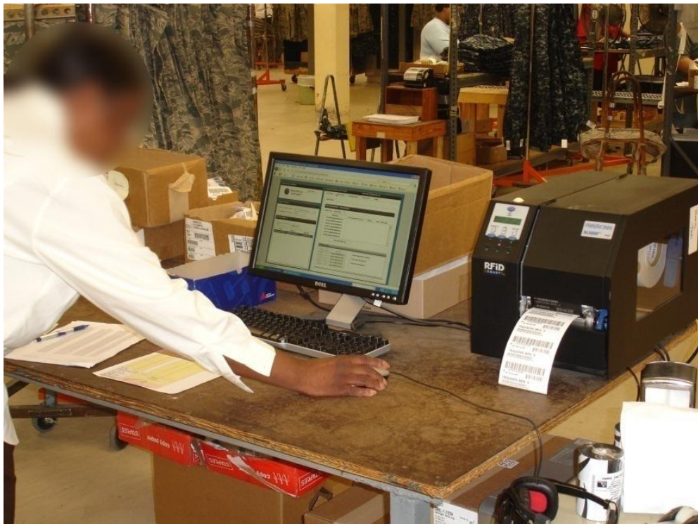
Figure 3. pRFID Item-Level Tags Encoded and Printed
