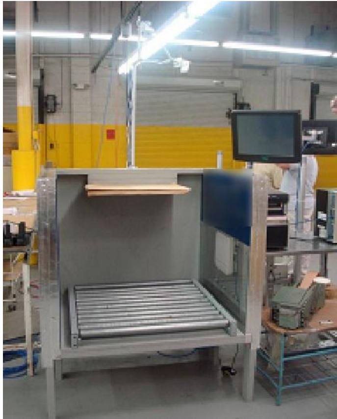
Figure 15. Conveyor with Fixed pRFID Readers
