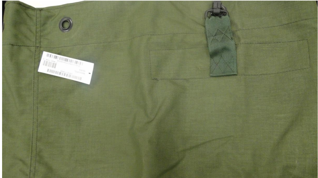
Figure 9. Attachment of pRFID Item Tag to Duffel Bags
