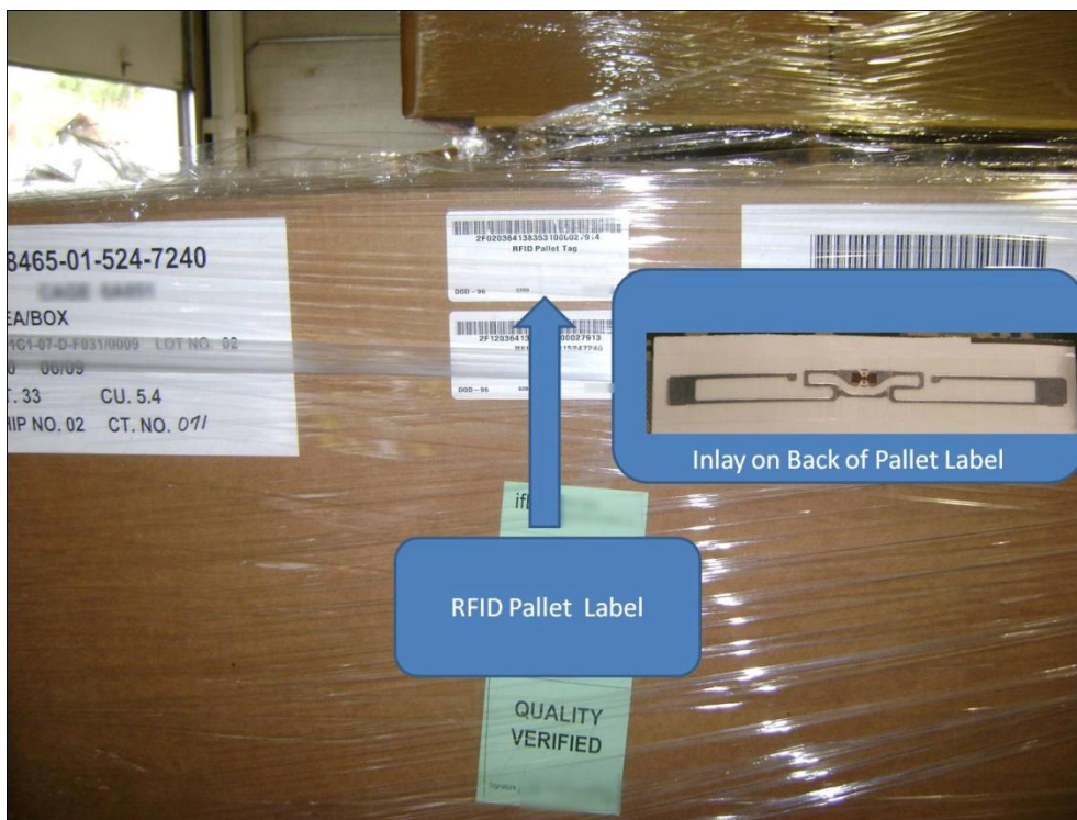
Figure 20. Pallet Label Attached to Pallet and Back of Pallet Label Showing Inlay
