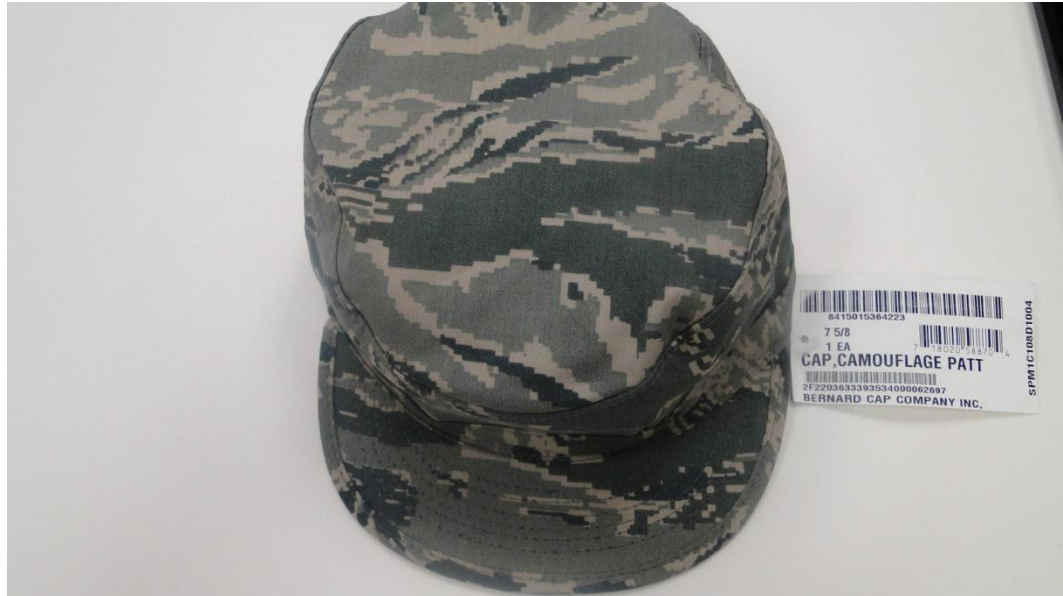
Figure 8. Attachment of pRFID Item Tag to Caps
