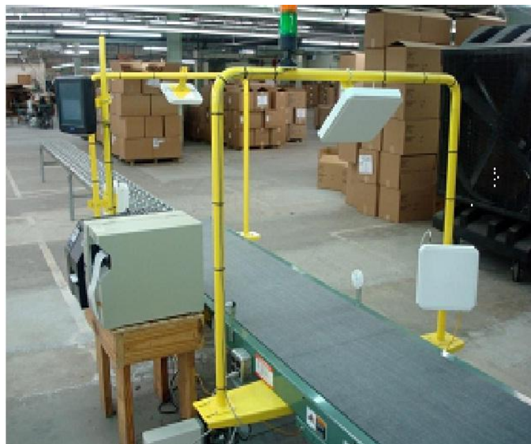
Figure 15. Conveyor with Fixed pRFID Readers
